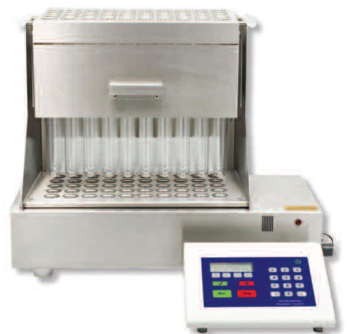
50 place block with digestion tubes in the cooling position
